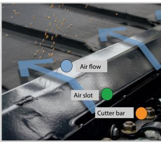
Air is blown in a consistent and controlled stream through the slots right behind the knife, carrying the grains and dropping them onto the belt.
