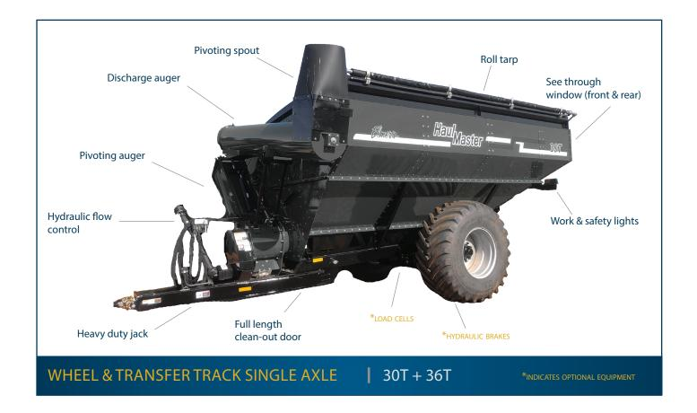
Elmer's Transfer Tracks are an available option on the 30T and 36T Haulmasters. Transfer Tracks increase fuel efficiency while reducing the impact on soils.
