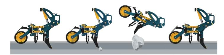
The assembly includes a semi-independent break away on the tines. Tines can clear small obstacles without changing the seed depth or press wheel downforce. When a larger obstacle is encountered, the entire assembly will trip to avoid damage. The hydraulic cylinder circuit is also equipped with a built-in damper accumulator, this allows for a controlled return of the tine after tripping. Breakout force is user adjustable for optimum performance, as required.
