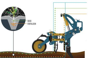
**Liquid fertiliser placement:** behind tine or seed Seed depth placement
